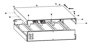
Once the battery box is opened, remove the two battery fixing plates present on the left side of the battery box by unscrewing the 4 screws present.
