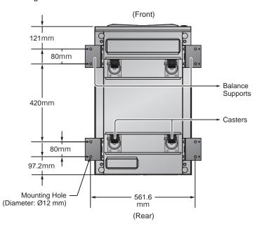
(Figure 6-3: Mounting Hole Diagram)
