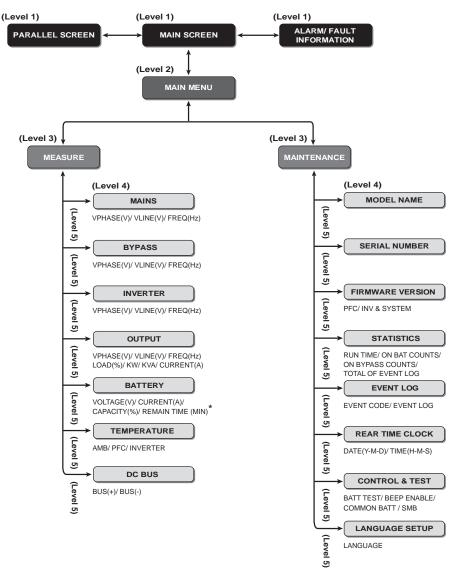
(Figure 8-1: LCD Display Hierarchy)
