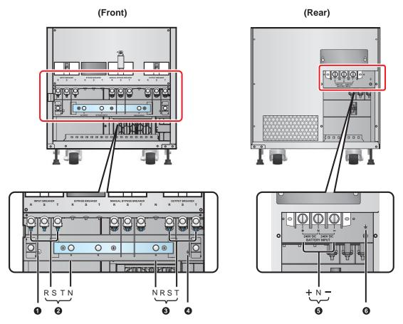
(Figure 6-7: 80kVA Model - Wiring Terminal Block)
