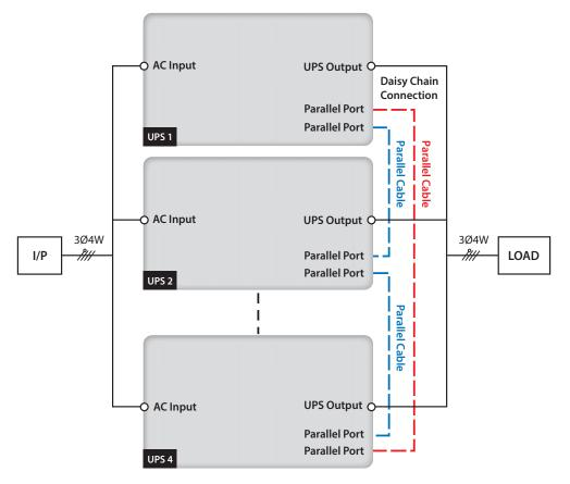
(Figure 6-15: Parallel Units Single Input Wiring Diagram)
