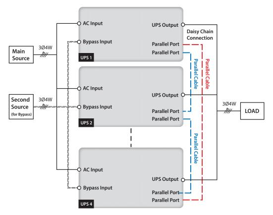
(Figure 6-16: Parallel Units Dual Input Wiring Diagram)
