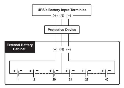
(Figure 6-17: External Battery Cabinet Connection )
