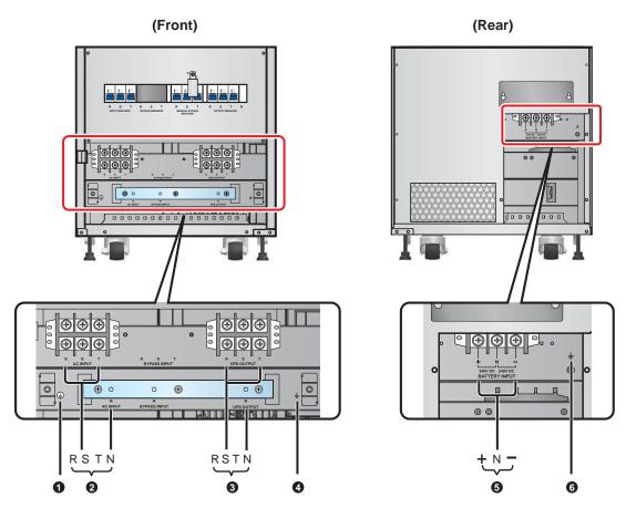
(Figure 6-6: 60kVA Model - Wiring Terminal Block)
