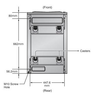
(Figure 6-2: UPS Cabinet Fixing Hole Diagram)
