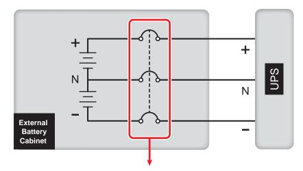
2) 3-pole DC circuit breaker (per pole voltage ≥500Vdc)
