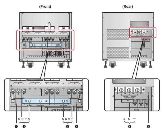
(Figure 6-8: 100/ 120kVA Model - Wiring Terminal Block)
