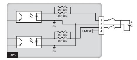
(Figure 5-9: Input Dry Contact Configuration II)
