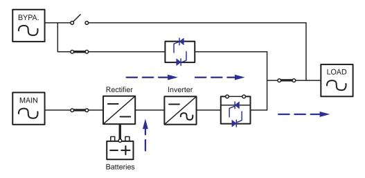
(Figure 4-4: Path of Electrical Power through the UPS in Battery Mode)
