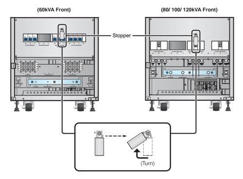
(Figure 7-1: Manual Bypass Breaker's Stopper Location)
