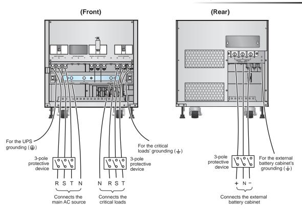
(Figure 6-11: 100/ 120kVA Model - Single Unit Single Input Wiring Diagram)
