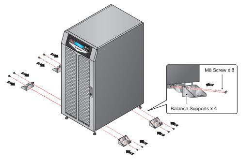
(Figure 6-4: Balance Support Installation)
