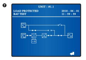
When the screen above appears, it means that the UPS is executing a battery test.
