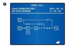
When the screen above appears, it means the bypass is supplying power to the critical loads.
