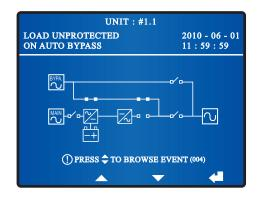
3 Turn on the Output Switch (Q4), the Output Switch LED **6** illuminates and the following screen appears. Now the bypass supplies power to the output.
