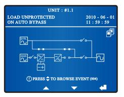
2 Turn on each unit's Output Switch (Q4). Each unit's Output Switch LED **6** o illuminates and each unit's LCD shows the following screen. At this moment, the bypass supplies power to the output.
