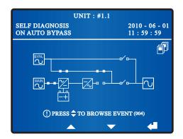
S After each unit's inverter voltage establishes, all parallel UPSs will transfer to normal mode. At this moment, each UPS's Inverter Power Supply LED I illuminates and each UPS's LCD shows the following screen.
