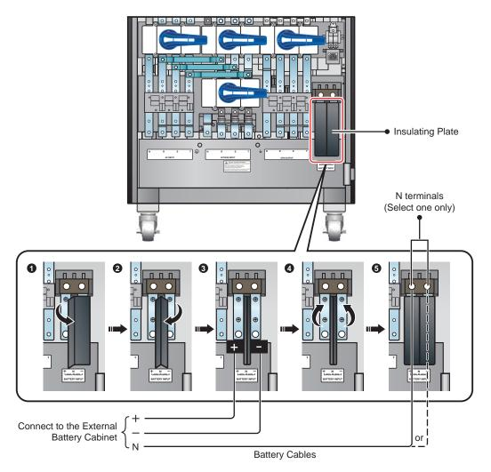
(Figure 5-18: External Battery Cabinet Wiring)
