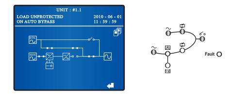
If the UPS that you turned off matches 1) situation, repeat the procedures stated in 1 to continually switch the remaining parallel UPSs into bypass mode.
