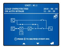
Press each UPS's ON button I for three to ten seconds and release it after you hear one beep. In the meantime, each unit's inverter starts up, each unit's Inverter Start-up LED ⊠ is on, each UPS is in bypass mode, and the following screen appears on each unit's LCD.
