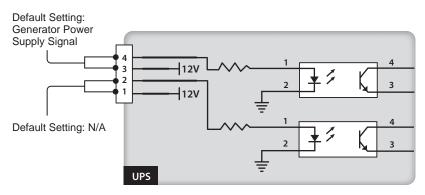
(Figure 4-2: Input Dry Contacts (Two Sets))
