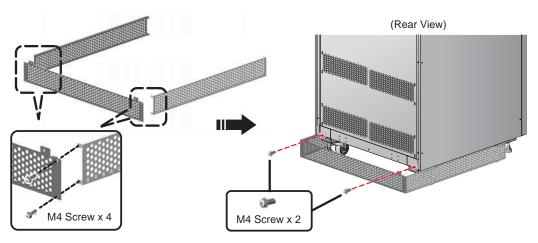
(Figure 5-3: Install the Rodent Shields at the Rear of DPS)
