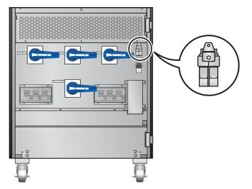
(Figure 6-1: Close the Auxiliary Power Fuse Holder)
