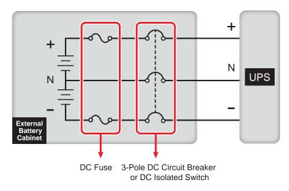
(Figure 5-20: Installation of a 3-Pole DC Circuit Breaker or DC Isolated Switch Connected in Series with a DC Fuse)
