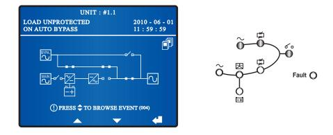
2 Turn off one of the parallel UPSs' Bypass Switch (Q2) and Output Switch (Q4), and the UPS's all LEDs and LCD are off. If you need to turn off the remaining parallel UPSs, please repeat the procedures above.
