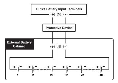
(Figure 5-17: External Battery Cabinet Connection)
