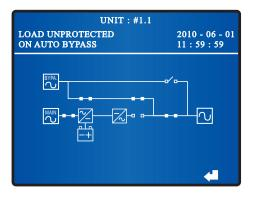
**5** Press the **ON** button **1** on the control panel for three to ten seconds and release it after you hear one beep. The following screen appears.
