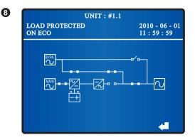
When the screen above appears, it means that the UPS is in ECO mode and the bypass supplies power to the critical loads. Please see **7.7.2** *Output Setup* for ECO mode setup.
