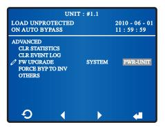
If you select **'SYSTEM'**, the UPS will upgrade system's firmware. If you choose **'PWR-UNIT'**, the UPS will upgrade power unit's firmware. After you select **'PWR-UNIT'**, the following screens appear in order.
