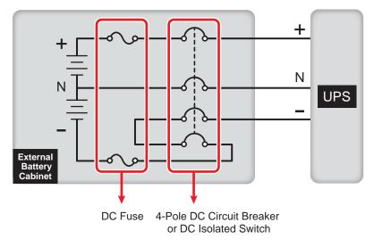
(Figure 5-19: Installation of a 4-Pole DC Circuit Breaker or DC Isolated Switch Connected in Series with a DC Fuse)
