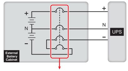
Option 3: Installation of a 4-pole DC circuit breaker (per pole voltage  $\geq$  250Vdc)
