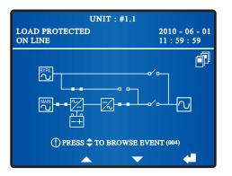
6 Measure each UPS's voltage difference between phases (should be below 5V). If normal, turn on each UPS's Output Switch (Q4). At this moment, each unit's Output Switch LED of o lights on and each UPS's LCD shows the following screen. If abnormal, please contact maintenance personnel.
