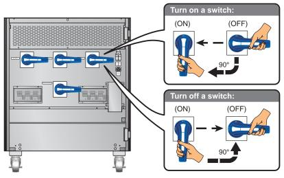
(Figure 2-9: Turn on/ off a Switch)
