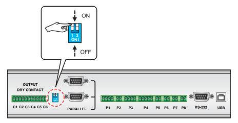
(Figure 6-3: Set up the Parallel Switch)
