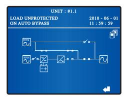
Turn on each UPS's Input Switch (Q1), each unit's Main AC Source LED ~ illuminates, and each UPS's LCD shows the following screen.
