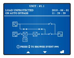
2 Turn on the Output Switch (Q4). The Output Switch LED **6** illuminates and the following screen appears. The bypass supplies power to the output.
