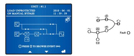
Turn off each UPS's Manual Bypass Switch (Q3). Per unit transfers into bypass mode, each UPS's LEDs illuminate without any change and each UPS's LCD shows the following screen.
