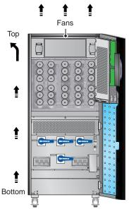
(Figure 5-1: Fan Ventilation Direction)
