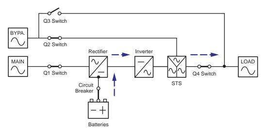
(Figure 3-2: Path of Electrical Power through the UPS in Battery Mode)
