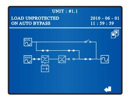
**6** Press each UPS's **ON** button **1** on the control panel for three to ten seconds and release it after you hear one beep. At this moment, each UPS's LEDs illuminate without any change and each unit's LCD shows the following screen.
