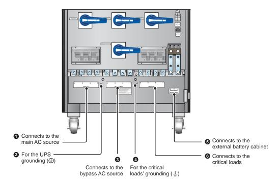
(Figure 2-13: Wiring Terminal Block)
