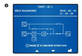
When the screen above appears, it means that batteries have started up the UPS.
