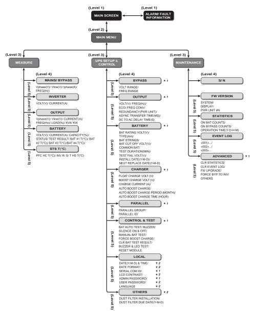
(Figure 7-1: LCD Display Hierarchy)
