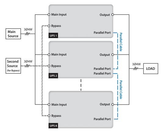
(Figure 5-16: Parallel Units Dual Input Wiring Diagram)
