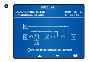
When the screen above appears, it means that the UPS is in manual bypass mode. Before maintenance, do not forget to switch the UPS into manual bypass mode and cut off the main AC source and batteries. During this mode, if the bypass AC source fails, the critical loads won't be protected.
