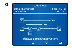
When the screen above appears, it means that the UPS is in battery mode.
