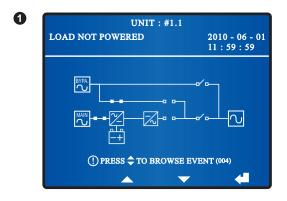
When the screen above appears, it means that no power is supplied to the critical loads connected.
