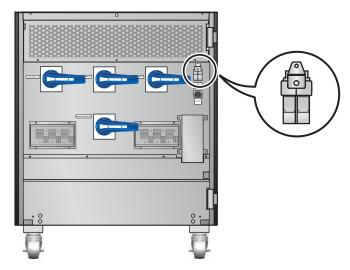
(Figure 6-2: Close the Auxiliary Power Fuse Holder)
