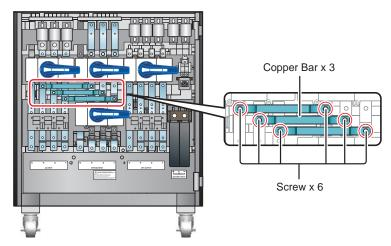
(Figure 5-10: Location of Six Screws and Three Copper Bars)
