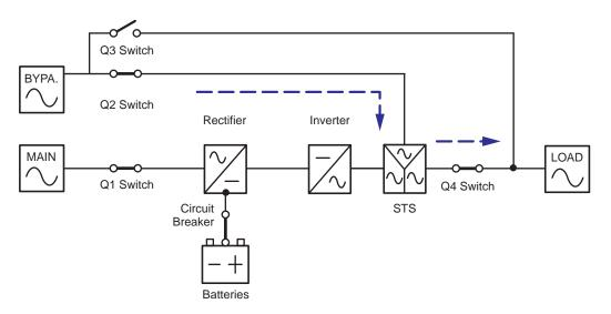
(Figure 3-3: Path of Electrical Power through the UPS in Bypass Mode)
