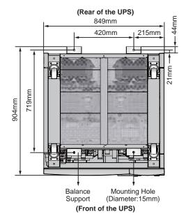
(Figure 2-3: Bottom View & Mounting Hole Diagram)
