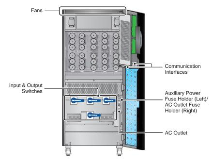
(Figure 2-5: Internal Mechanisms)
