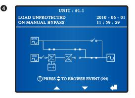
When the screen above appears, it means that the UPS is in bypass mode. If the bypass AC source fails, the critical loads won't be protected.
