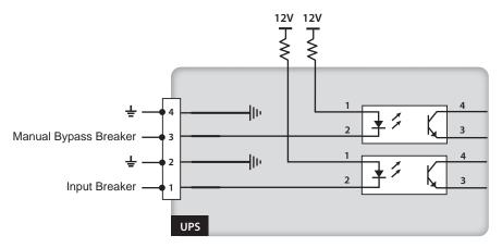
(Figure 4-4: Dry Contacts for External Breakers)
