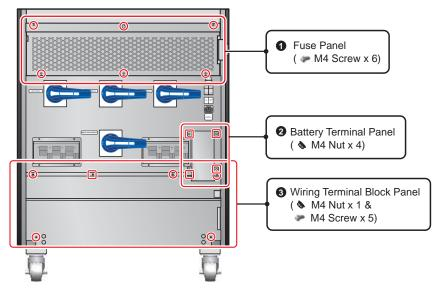
(Figure 5-7: Remove the Three Panels)
