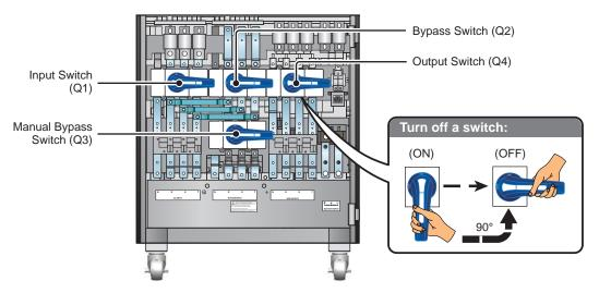
(Figure 5-12: Switch Location and Turn off a Switch)
