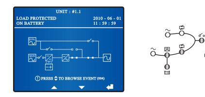
**1** During battery mode, the following screen appears and LEDs illuminate as follows.
