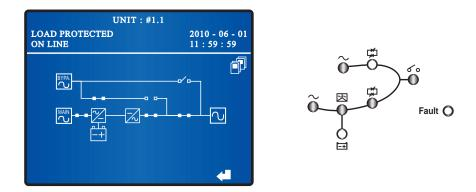
2) If the total critical loads exceed the remaining parallel UPSs' total capacity, all of the parallel UPSs' inverters will shut down, inverter static switches will automatically turn off, and all parallel UPSs will transfer to bypass mode. The total critical loads will be shared equally by all parallel UPSs, and the status of LCD and LEDs for each of the parallel UPSs is as follows.
