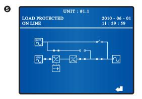
When the screen above appears, it means that the UPS is in normal mode.
