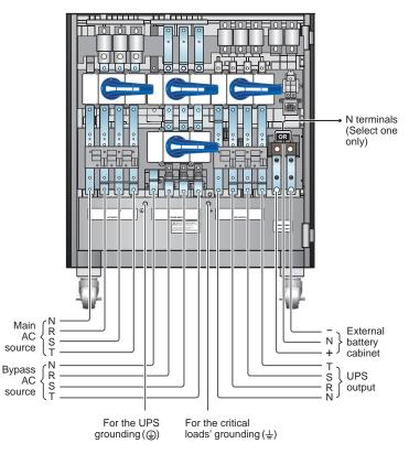
(Figure 5-14: Single Unit Dual Input Wiring Diagram)
