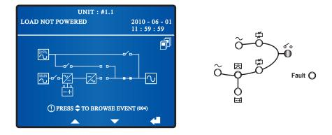
The status of the LCD and LEDs for the UPS that you turned off:
