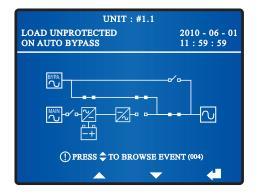
The nine statuses of the UPS shown in the LCD display are as follows.
