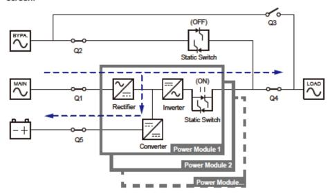
(Figure 3-1: On-Line Mode Diagram)
