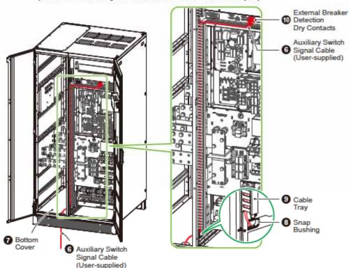
(Figure 4-14: Bottom Entry\_Auxiliary Switch Signal Cable Routing)
