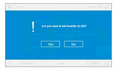
After selection of 'YES' to start up the UPS's inverter, the UPS will perform self-inspection, the system will begin synchronization with the bypass AC source and the tri-color LED indicator will remain yellow.
