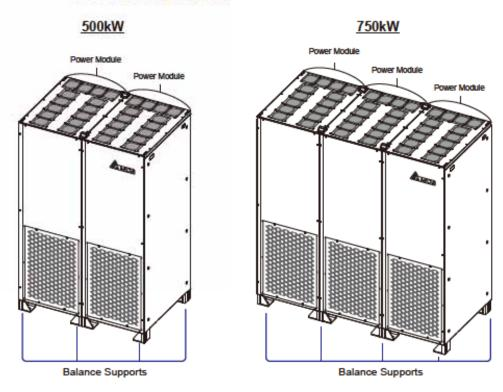
(Figure 2-11: Front View of the Power Modules)
