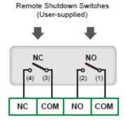
(Figure 4-29: REPO Dry Contacts\_ Pins' Location and Wiring Diagram)
