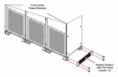
(Figure 5-17: Face the Front of the Power Modules & Install the Rodent Shield F at the Right Bottom Side)
