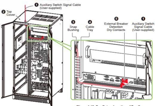
(Figure 4-12: Top Entry\_ Auxiliary Switch Signal Cable Routing)
