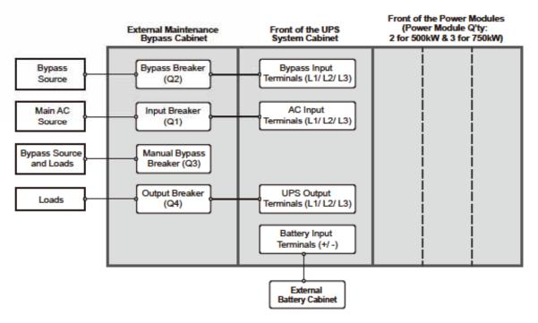
(Figure 5-33: Single Unit Dual Input Wiring Diagram)
