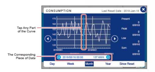
(1) Take the figure above as an example; if you tap the curve '2018-08-16', the data bar that shows the corresponding piece of data will appear below the chart and show the kWH statistics '137 kWH' of the UPS main input of the day.
