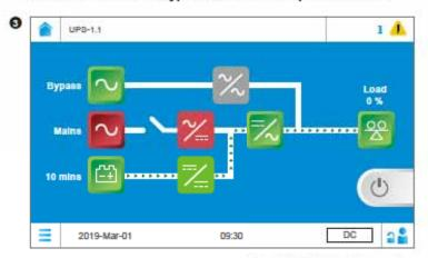
The screen above indicates that the UPS is in DC mode, and power supply of the loads comes from the batteries. Please refer to 6.2.2 Battery Mode Start-up Procedures.
