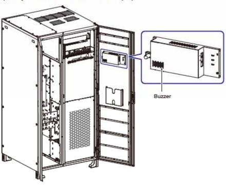
(Figure 2-18: Buzzer Location)
