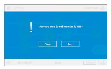
After selection of 'YES', the UPS's inverter will start up, the UPS will perform self-inspection, the system will begin synchronization with the bypass AC source and the tri-color LED indicator will remain yellow.
