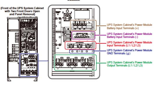
(Figure 2-9: Wiring Terminals inside the UPS System Cabinet)
