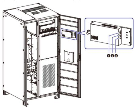
(Figure 4-31: Communication Interfaces \_ at the Rear of the Touch Panel)
