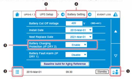
(Figure 4-27: Battery Charging Protection (IP DRY 2) Setup)
