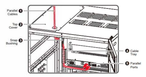
(Figure 5-37: Top Entry & Location of Parallel Cables, Top Cover, Snap Bushing, Cable Tray and Parallel Ports)
