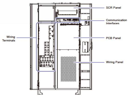
(Figure 2-8: Internal View of the UPS System Cabinet with Two Front Doors Open)
