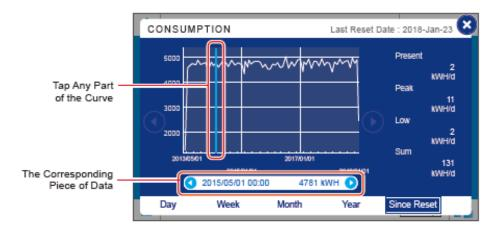
(1) Take the figure above as an example; if you tap the curve '2015-May', the data bar that shows the corresponding piece of data will appear below the chart and show the kWH statistics '4781 kWH' of the UPS main input of the month.
