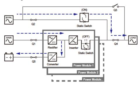
(Figure 3-5: ECO Mode Diagram)
