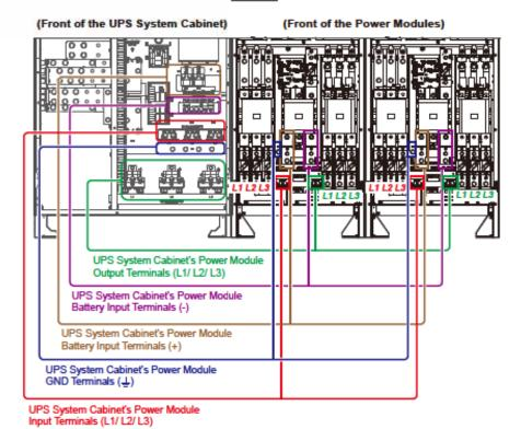
(Figure 5-26: Internal Wiring between the UPS System Cabinet and the Power Modules \_ 500kW UPS)
