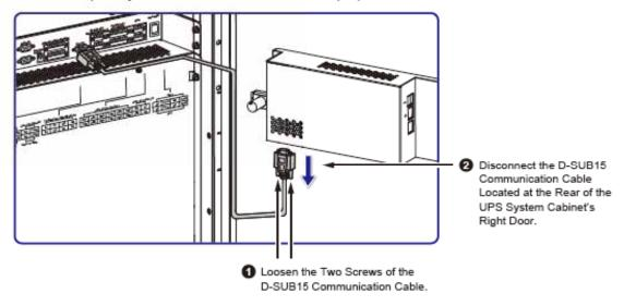
(Figure 9-2: Disconnect the D-SUB15 Communication Cable Located at the Rear of UPS System Cabinet's Right Door)
