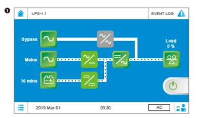
The screen above indicates that the UPS is in AC mode, and power supply of the loads comes from the inverter. Please refer to 7.9.2 Mode Setting and 6.2.1 On-Line Mode Start-up Procedures.
