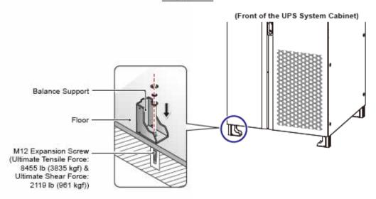
(Figure 5-8: Balance Support Installation Method for the UPS System Cabinet)
