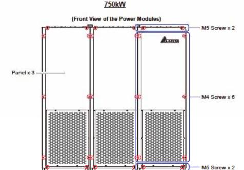
(Figure 5-12: Location of the Power Modules' Front Panels & Screws)
