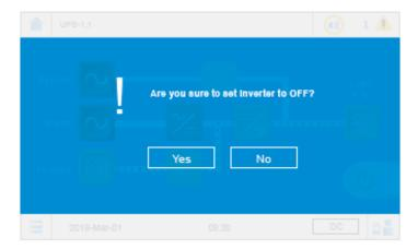
After selection of 'YES', the inverter will shut down, and the UPS will stop supplying power to the connected loads and start up shut-down procedures. About 3 ~ 5 minutes, the green inverter icon becomes grey and the tri-color LED indicator remains yellow.
