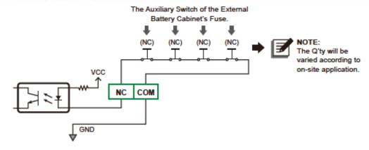
(Figure 4-21: Battery Fuse Detection Dry Contacts Pins' Location and Wiring Diagram)
