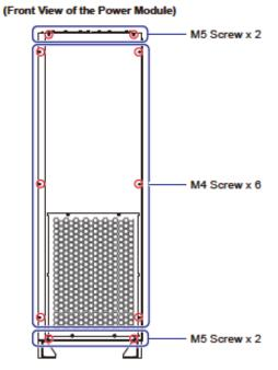
(Figure 5-24: Removal of Every Power Module's Front Panel)
