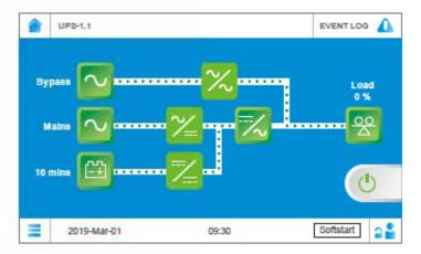
After the self-inspection and synchronization are both completed, the UPS will automatically transfer from bypass to inverter and let the inverter supply power to the connected loads. After the online mode start-up procedures are completed, the LCD will show the following screen and the tri-color LED indicator will illuminate green.
