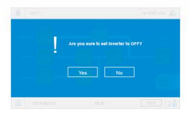
After selection of 'YES', the inverter will shut down. Now, the bypass source supplies power to the connected loads and the tri-color LED indicator illuminates yellow.
