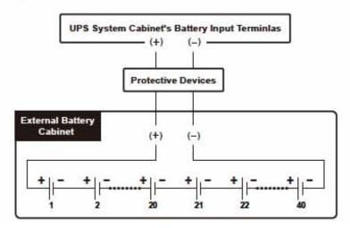
(Figure 5-42: External Battery Cabinet Connection)
