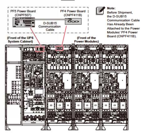
(Figure 5-13: Connect the D-SUB15 Communication Cable to the UPS System Cabinet's PF5 Power Board (CNPF507))
