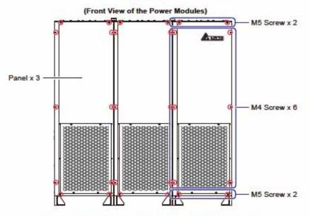
(Figure 2-12: Location of the Power Modules' Front Panels & Screws)
