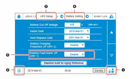
(Figure 4-28: Battery Fault Alarm (IP DRY 1) Setup)
