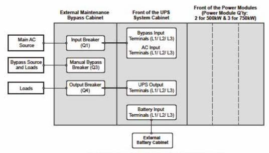
(Figure 5-31: Single Unit Single Input Wiring Diagram)
