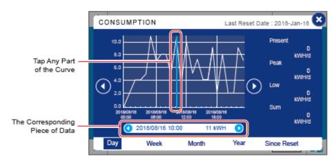
(1) Take the figure above as an example; if you tap the curve '2018-08-16 10:00', the data bar that shows the corresponding piece of data will appear below the chart and show the kWH statistics '11 kWH' of the UPS main input from 10:00 ~ 11:00 on that date.
