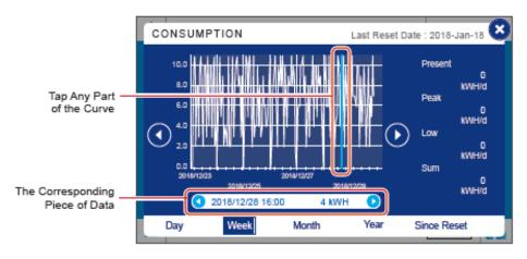
(1) Take the figure above as an example; if you tap the curve '2018-12-28 16:00', the data bar that shows the corresponding piece of data will appear below the chart and show the kWH statistics '4 kWH' of the UPS main input from 16:00 ~ 17:00 of that date.
