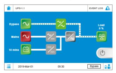
Next, turn OFF the external maintenance bypass cabinet's output breaker (Q4) and each external battery cabinet's breaker (Q5). At this moment, the tri-color LED indicator still illuminates yellow.
