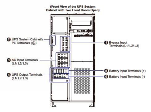
(Figure 5-30: Wiring Terminals of the UPS System Cabinet)
