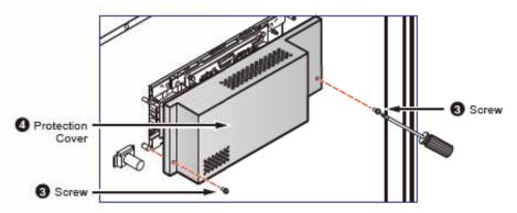
(Figure 9-3: Remove the Protection Cover Located at the Rear of the UPS System Cabinet's Right Door)
