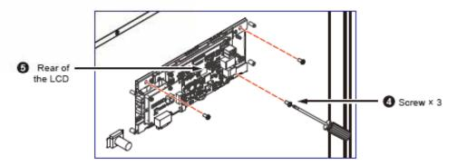
(Figure 9-4: Remove the Three Screws from the Rear of the LCD)
