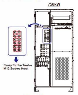
(Figure 5-21: Firmly Fix the M12 Screws)
