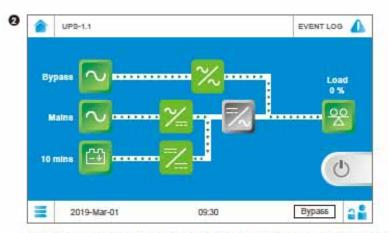
The screen above indicates that the UPS is in Bypass mode and the inverter is off. Please refer to 6.2.3 Bypass Mode Start-up Procedures.
