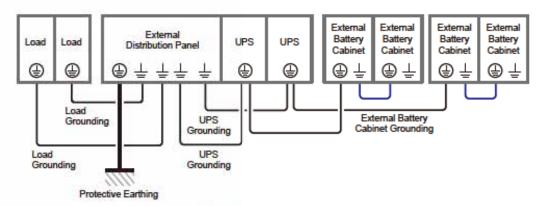
(Figure 5-40: Grounding Diagram\_ Parallel Units)
