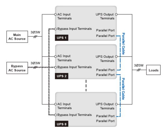
(Figure 5-41: Parallel Units Dual Input Wiring Diagram)
