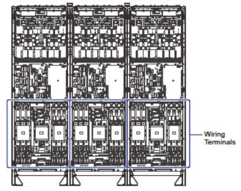
(Figure 2-13: Location of the Power Modules' Wiring Terminals)
