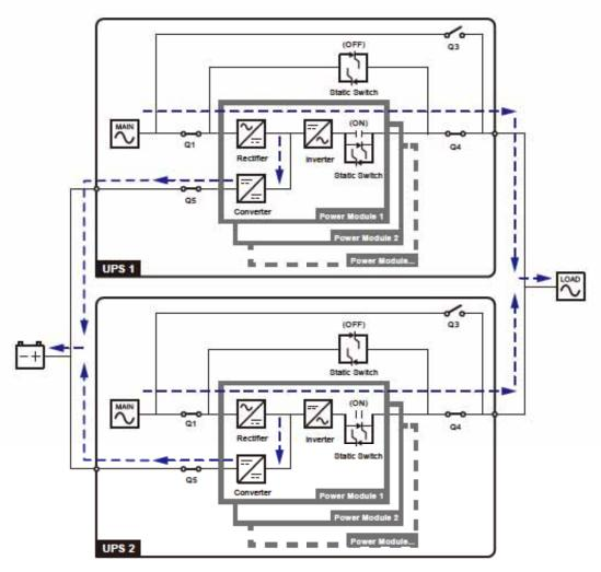
(Figure 3-7: Common Battery Diagram\_ only for Parallel UPSs Connecting to the Same External Battery Cabinet(s))
