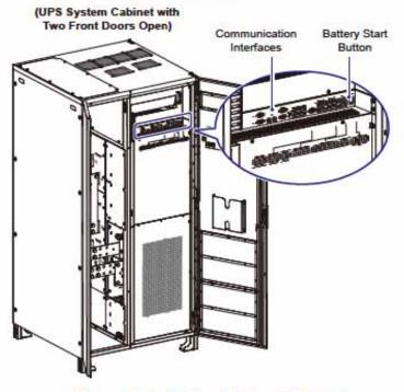
(Figure 7-2: The Position of Battery Start Button)
