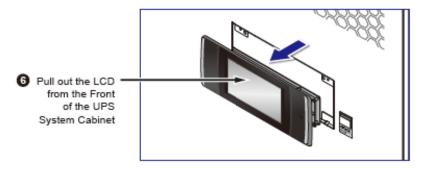
(Figure 9-5: Pull Out the LCD from the Front of the UPS System Cabinet)
