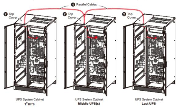
(Figure 5-36: Top Entry\_ Parallel Cables Routing)
