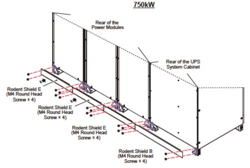
(Figure 5-15: Install the Rodent Shields at the Rear Bottom of the UPS System Cabinet and the Power Modules)
