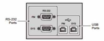
(Figure 4-7: RS-232 Ports & USB Ports)
