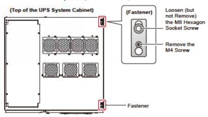
(Figure 5-4: Remove the Two M4 Screws & Loosen the Two M8 Hexagon Socket Screws of the Two Fasteners Located on the Top of the UPS System Cabinet)
