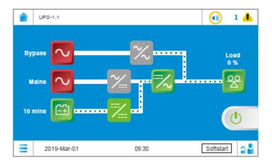
After the DC BUS voltage is established, the inverter will start up and the UPS will perform self-inspection. Now, tap the Main Menu icon
