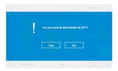
After selection of 'YES', the invert will shut down and stop running. Next, the UPS will transfer from inverter to bypass and let the bypass source to supply power to the connected loads, and the tri-color LED indicator will illuminate yellow.
