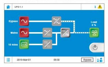
Next, switch OFF the external maintenance bypass cabinet's output breaker (Q4) and each external battery cabinet's breaker (Q5). Then, the LCD and the tri-color LED indicator are both off.
