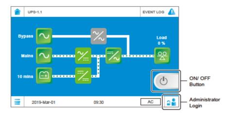
(Figure 7-5: Main Screen Administrator Login & ON/ OFF Button Location)
