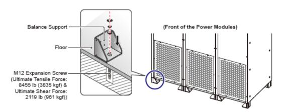
(Figure 5-9: Balance Support Installation Method for the Power Modules)
