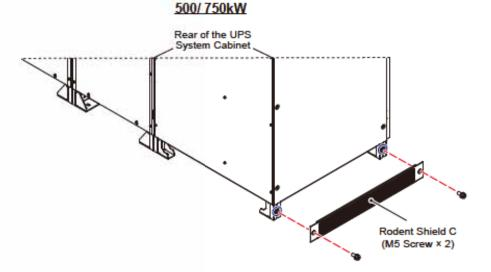
(Figure 5-16: Face the Rear of the UPS System Cabinet & Install the Rodent Shield C at the Right Bottom Side)
