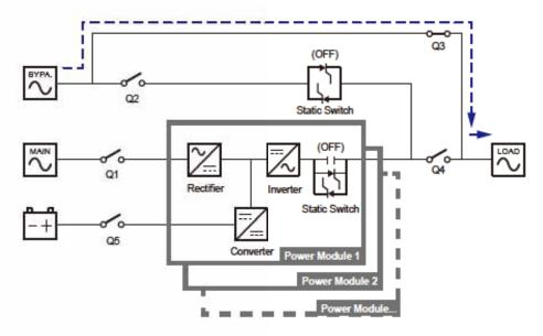
(Figure 3-4: Manual Bypass Mode Diagram)
