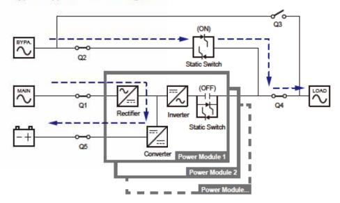
(Figure 3-3: Bypass Mode Diagram)
