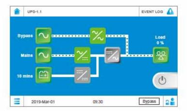
After the DC BUS voltage is established, the charger converter will start up and begin to charge the batteries. Meanwhile, it will be the bypass source to supply power to the connected loads.
