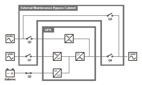
(Figure 3-2: Dual Input Application\_ UPS & External Maintenance Bypass Cabinet's Structure)
