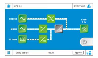
Tap the Main Menu icon = located in the lower left corner of the LCD and select UPS Setup → Mode Setting → On-Line. Next, the following screen appears.
