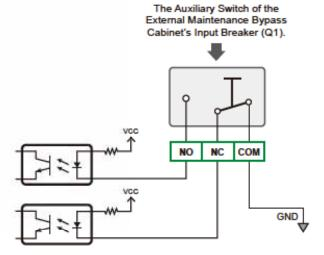
(Figure 4-19: Input Breaker Detection Dry Contacts Pins' Location and Wiring Diagram)
