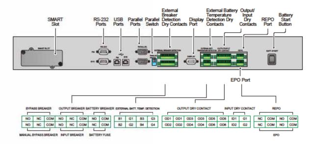
(Figure 4-2: Communication Interfaces on the Front of the UPS System Cabinet with Two Front Doors Open)
