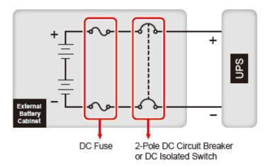
(Figure 5-43: Installation of a 2-Pole DC Circuit Breaker or DC Isolated Switch Connected in Series with a DC Fuse)
