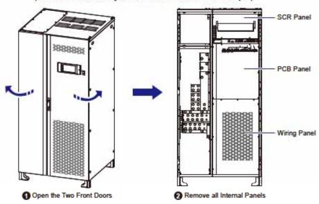
(Figure 5-22: Internal Panels Location of the UPS System Cabinet)
