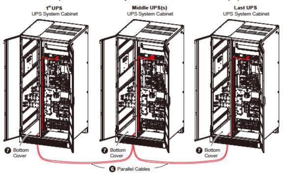
(Figure 5-38: Top Entry\_ Parallel Cables Routing)
