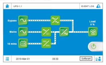
After the self-inspection and synchronization are both completed, the UPS will automatically transfer from bypass to inverter and let the inverter supply power to the connected loads. Once the manual bypass mode transferring to online mode procedures are completed, the LCD will show the following screen and the tri-color LED indicator will illuminate green.
