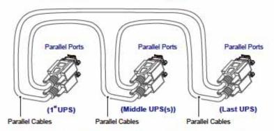
(Figure 5-35: Parallel Ports Connection among the Parallel UPSs)
