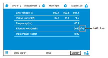
Tap the kWH icon , and you can check the kWH statistics of the UPS main input in the following window.
