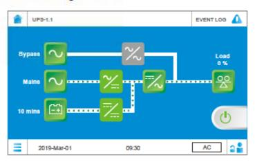
When bypass input voltage and frequency are within the range of rating voltage ±10% and rating frequency ±5Hz, it will be bypass power to supply power to the connected loads. If out of the above mentioned range, it will be the inverter to supply power to the loads. In ECO mode, the tri-color LED indicator illuminates green.
