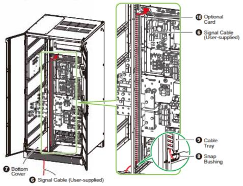
(Figure 4-5: Bottom Entry\_ Optional Card's Signal Cable Routing)
