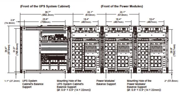
(Figure 5-7: Mounting Hole Diagram)
