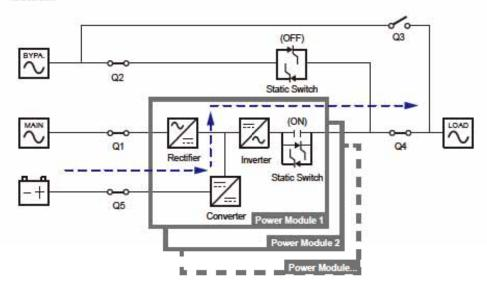
(Figure 3-2: Battery Mode Diagram)
