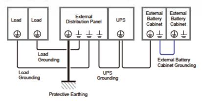
(Figure 5-32: Grounding Diagram\_ Single Unit)
