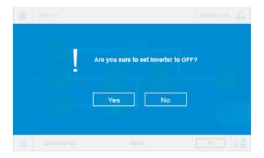
After selection of 'YES', the inverter will shut down. At the same time, the UPS will transfer from inverter to bypass and let the bypass source supply power to the connected loads, and the tri-color LED indicator will illuminate yellow.
