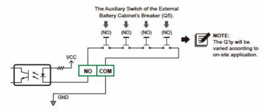
(Figure 4-20: Battery Breaker Detection Dry Contacts\_ Pins' Location and Wiring Diagram)
