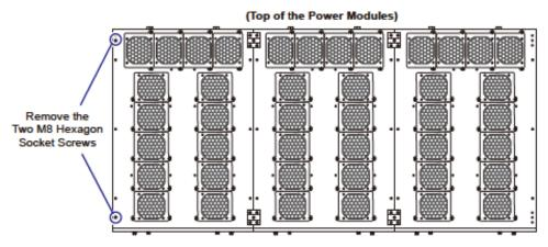
(Figure 5-5: Remove the Two M8 Hexagon Socket Screws Located on the Top of the Power Modules)
