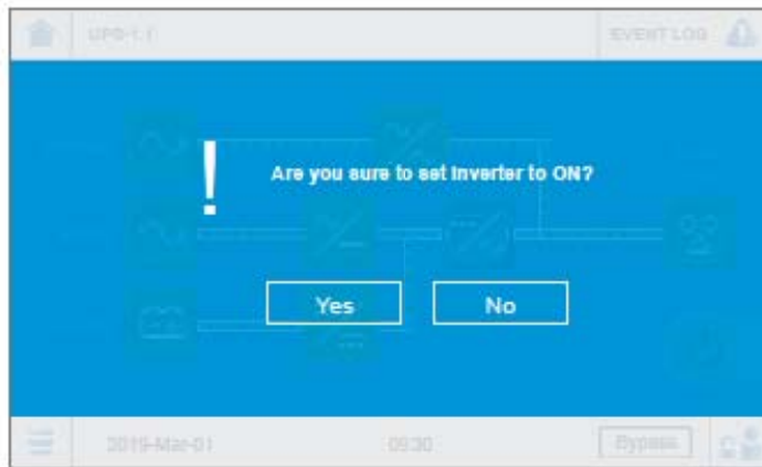
(Figure 7-6: Power on Reminder Window)
